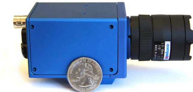
Nuvation's IP Camera Reference Design featuring TI DaVinci™ Technology
