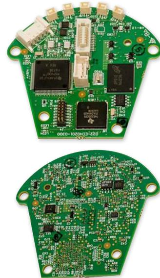
Custom smart leak detector for monitoring fire hydrants, developed by Nuvation Engineering. Hydrants are connected through a proprietary mesh network.
