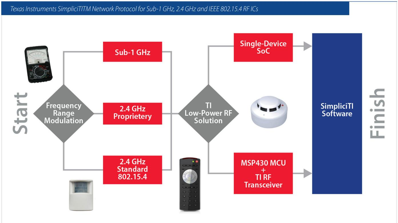
TI SimpliciTI™ is a low-power RF protocol aimed at simple, small RF networks. This open-source software is an excellent start for building a network with battery-operated devices using one of TI's low-power RF System-on-Chips (SoC) or the MSP430 ultra-low-power MCU and a TI RF transceiver.
